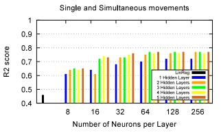
Fig. 2: Breakdown of test  $R^2$  scores for different network topologies, standard Hudgins features, corpus with and without simultaneous movements. Averaged over development subjects.
