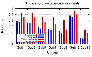
Fig. 3: Breakdown of  $R^2$  scores on training and test subsets for different subjects and two network topologies (small: one hidden layer with 32 neurons, reference: three hidden layers with 128 neurons), standard Hudgins features, corpus with and without simultaneous movements.
