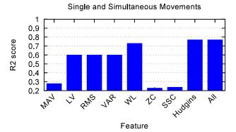
Fig. 4:  $R^2$  scores on different single features, as well as on the standard Hudgins feature set and an extended feature set (see section III for details), using the reference NN architecture. Averaged over development subjects.
