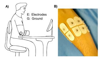
Fig. 1. Experimental setup. A) Participants sat on a chair with the elbow flexed at 90° on a cushion wearing a matrix of EMG electrodes and looking at a computer screen. The latter displayed in real time a biofeedback signal proportional to the average mean absolute value across the channels. B) Placement of the EMG electrodes around the forearm.
