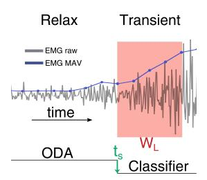
Fig. 2. Transient EMG classifier components. Once the Onset Detection Algorithm (ODA) identifies an onset (at t<sub>s</sub>), the portion of EMG MAV (Mean Absolute Value) within the window W<sub>L</sub> is extracted and fed to the classifier.
