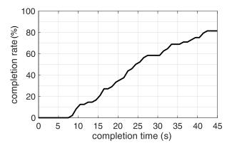
Fig. 7. TAC test performance of the amputee participant (i.e, A1). The curve indicates the percentage of trials completed in a certain amount of time.
