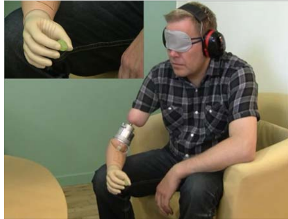
Figure 1. Osseointegrated human-machine gateway (OHMG) providing bidirectional communication between the self-contained artificial limb controller (ALC) and implanted neuromuscular interfaces. The patient is capable to grab a grape blindly by receiving direct neural information from sensory embedded in the thumb of the hand.
