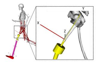
Figure I. Visual representation of the scaled full body musculoskeletal model of a TFA with the local coordinate system for the bone-implant interface indicated. The pink dots represent the virtual markers and the red lines represent the geometric paths of the muscles included in the model.
