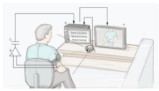
**Figure 2** Schematic illustration of the clinical investigation device with all its components. Myoelectric signals are acquired though surface electrodes (A) by a myoelectric amplifier (B), electrically isolated (C). The signals are then processed by the software installed on the computer (D). The camera (E) films the participant and the recorded image is displayed on the monitor (F) with a virtual limb superimposed where the marker (G) is detected. Figure courtesy of Jason Millenaar.
