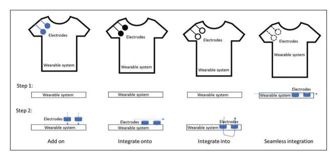
Figure 6. Wearable system integration levels.
