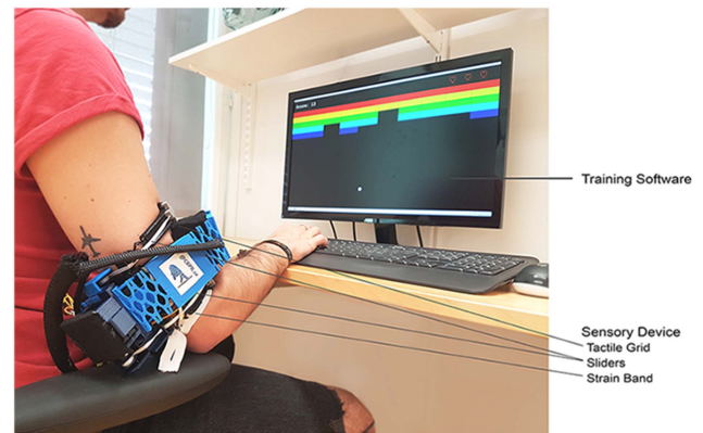
Fig. 5. Wearable somatosensory device for training tactile sensitivity.
