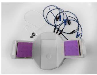
**Figure 1** Sensorimotor training device: a myoelectric acquisition system with two grids (vibrotactile display) to produce mechanosensory stimulation.
